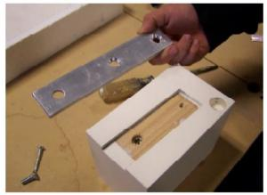
After the bracket is removed it will expose an embedded wood structure with one of the screw holes showing inserted 5/16" metal threads. These threads can be used to secure sculptures without exposed brackets if desired. Which is covered later in this information.
