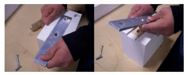
Grab the bracket and with firm leverage pop the bracket free from the fitted slot. You can us a hammer to tap the bracket loose if necessary.
